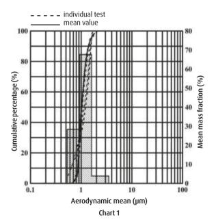
Test with Ventolin at normal temperature of 24 ±2°C, relative humidity: 45–75% and pressure: 86 kPa to 106 kPa, – for details: chart 2:
