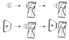
3.4.2. Attach the mouthpiece (installation directly onto the medicine cup connecting tube)
